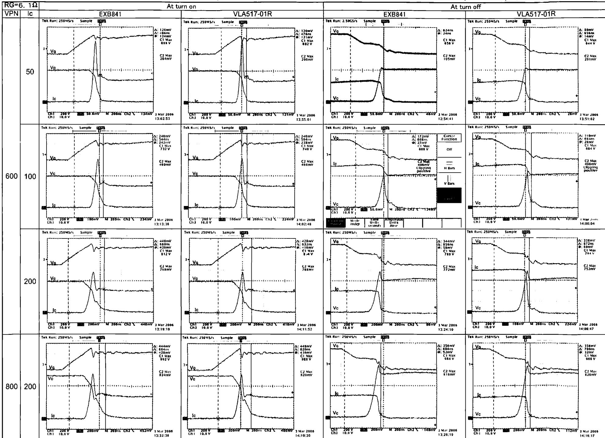
Ch3: VGE: 10V / DIV, Ch1: VCE: 200V / DIV, Ch2: Ic: 50 mV / DIV => 25A / DIV, 100mV => 50A, 200mV => 100A
